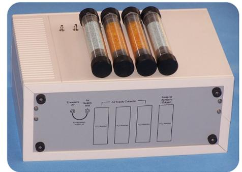
Self-indicating desiccants for analyzer zeroing and CO<sub>2</sub>/H<sub>2</sub>O control
