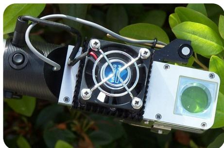
Close-up of PLC4 (B) leaf cuvette head
