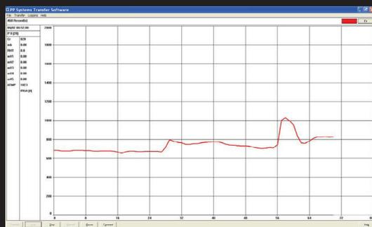
The EGM-4 is supplied with a Windows® based software program for transferring and logging sensor data. The sensor data may be recorded manually or automatically depending on user specified settings. Stored records (ASCII) can be later imported into your favorite spreadsheet program for further analysis.
